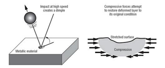
Each shot acts as a mini ball peen hammer striking the surface and forming a tiny dimple. The material below the surface tries to counteract the strain resulting in a layer of cold worked metal stressed in compression.
